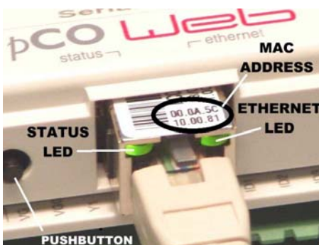
Figure 2.e - MAC address and indicator LEDs
