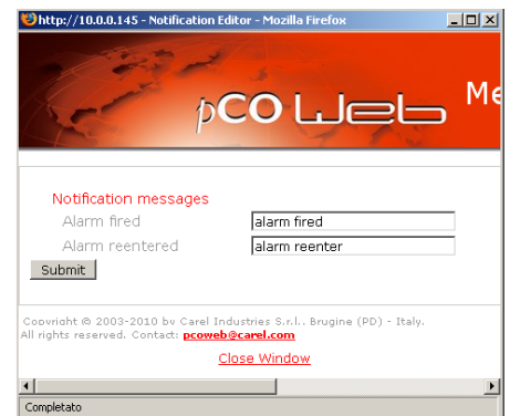
Figure 4.r – Setting the strings sent for Activation - Return
